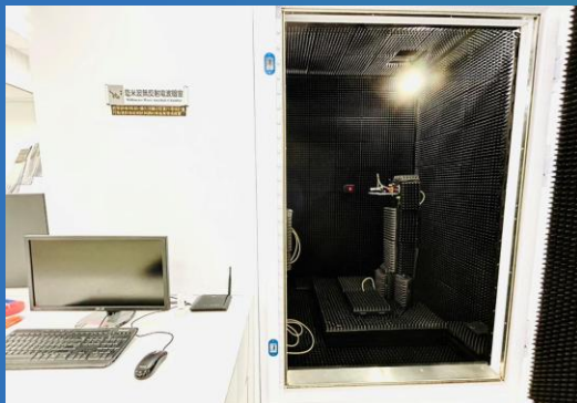
5G Mobile Communication Product Engineering Verification Laboratory – Millimeter Wave Non-Reflective Radio Wave Chamber
