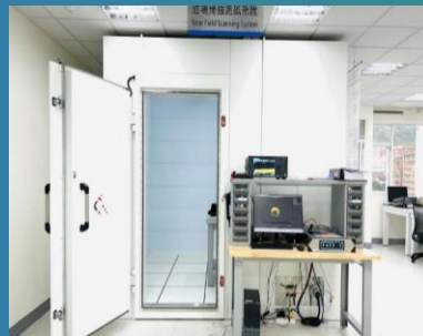
Near Field Scanning System
